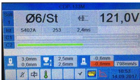
photo 1, above: way-measurement with process monitoring system
